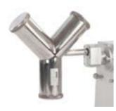
The Mixer Y5 with Y-shaped mixing vessel for the gentle mixture of solid well flowing materials (bulk materials). The rotary motion of the mixing vessel makes a particularly homogenous mixture possible and hence the device is suitabe for sensitive materials.
