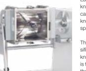
Laboratory Kneader with stainless steel capacity 65%) housing two z-shaped kneading blades running at different speeds in opposing directions.
