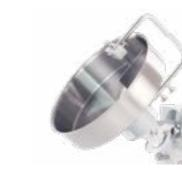
The pelletizer GTE (300 mm diameter) is of the requisite amount of liquid, this attached to the AR 403 via the Universal Gear UG which enables the opera- mation of pellets. The angle of the pan tor to adjust the operating angle to the and the amount of liquid added deteroptimal position during operation.
