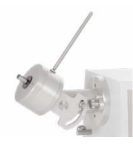
The new Universal Gear uses a modernised CNC machined aluminium design for improved durability. It is required for adjusting the angle of operation (±40°) and reduction of speed (1:5,75).
