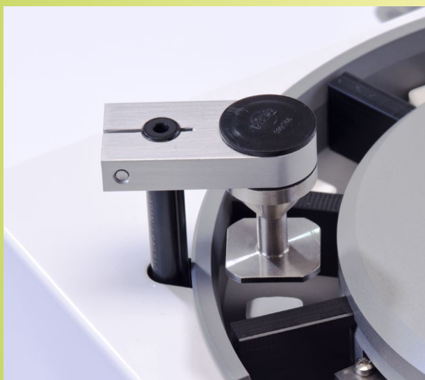
Optional thickness testing via a linear potentiometer*.
